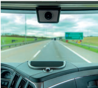
ABOVE: From July 2026, all new EU trucks must include camera-based driver monitoring systems to detect distraction
