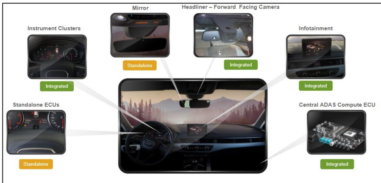
**Figure 1: Overview of landing points for DMS Processors and Optics**
